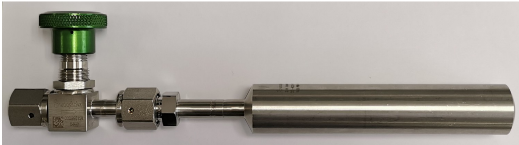
Single valve cylinder for dry box atmosphere sampling
